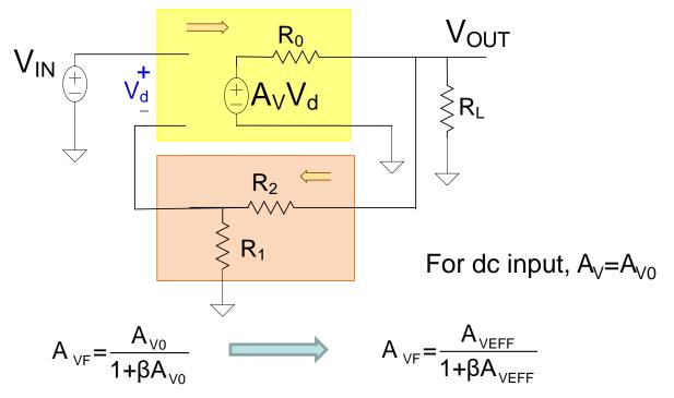
The open loop gain of an operational amplifier used in a FB configuration must include the loading of the feedback network and load resistor
