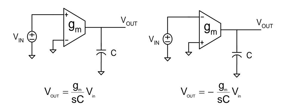
Noninverting Voltage Controlled Integrator
