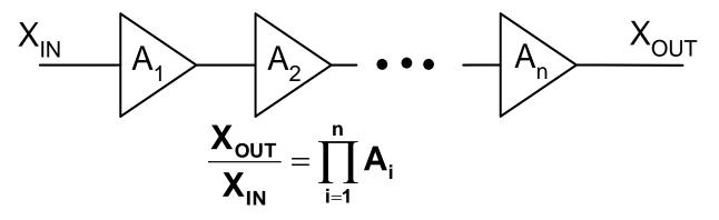
But each of the gains will roll off with frequency so can be modeled as
