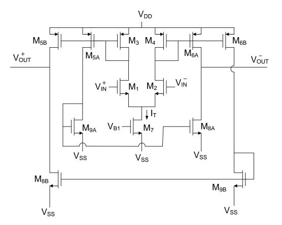
Need CMFB circuit and requires modest circuit modification to provide CMFB insertion point
