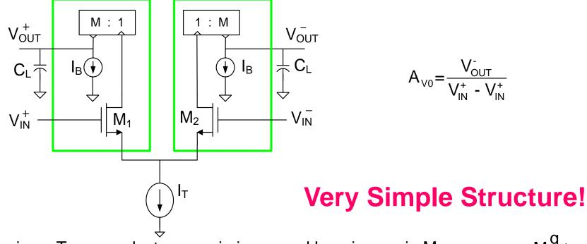
Premise: Transconductance gain increased by mirror gain M
