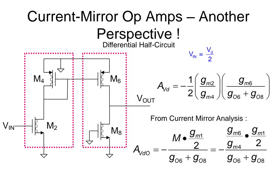
Cascade of n-channel common source amplifier with p-channel common-source amplifier !
