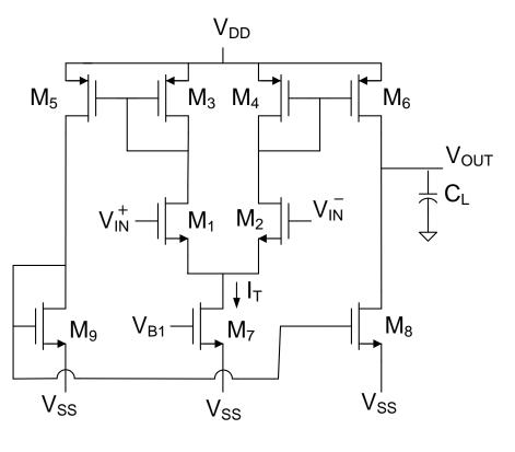
And can use higher output impedance current mirrors to decrease g<sub>OEQ</sub>
