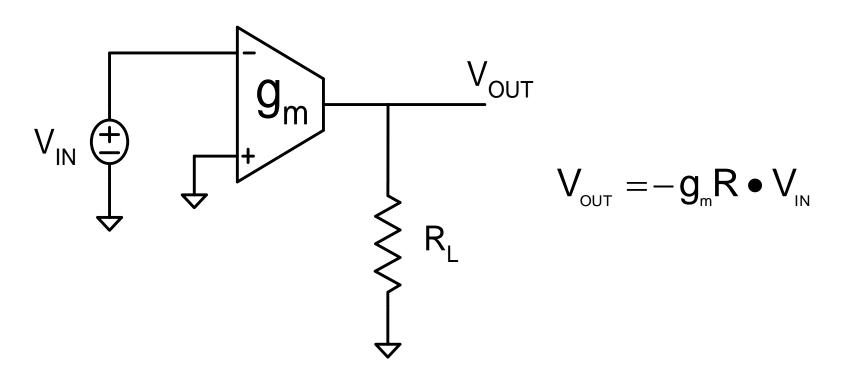
Voltage Controlled Inverting Amplifier
