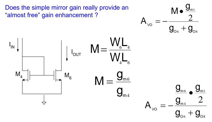
Gain Enhancement Potential Less Apparent but still Improved by  $g_{m6}/g_{m4}$  ratio
