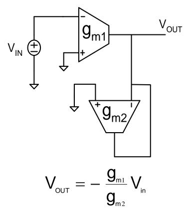
Inverting Voltage Controlled Amplifier
