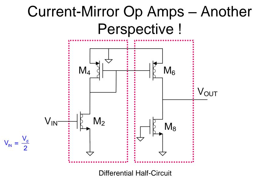
Cascade of n-channel common source amplifier with p-channel common-source amplifier !
