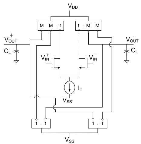
Need CMFB circuit and requires modest circuit modification to provide CMFB insertion point
